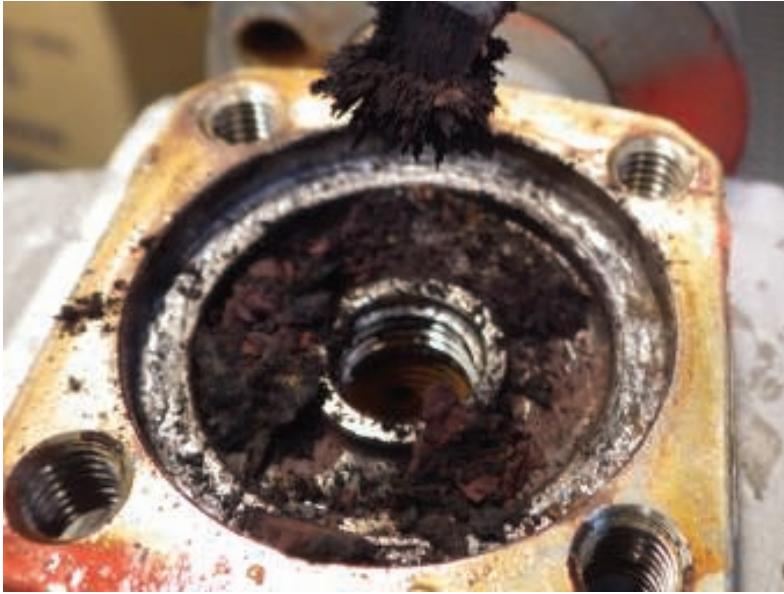
FIGURE 1. In the presence of oxygen, ferric-oxide corrosion occurs, and can wreak havoc on condensate-system equipment
