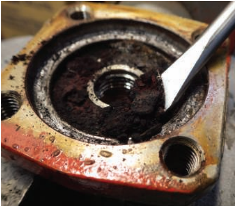
FIGURE 2. Corrosion in pipe walls can lead to widespread issues, including the formation of deposits and blockages in small piping components
