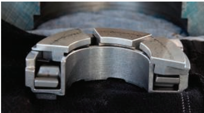
FIGURE 2. Tilting pad thrust bearings are widely used in relatively high-speed rotating machinery. These bearings are vulnerable and can be damaged easily; shown here is one that was removed for repair
